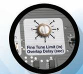
Innovative fine tune adjustment for the end of gate travel ( down to 1/8")
